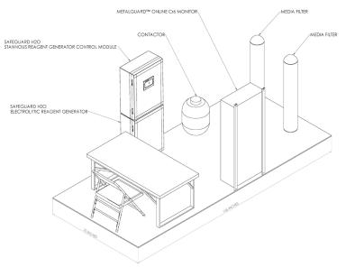
SafeGuard<sup>™</sup> H2O Cr6 Removal Demonstration Trailer comprises five main components: the stannous reagent generation control module, electrolytic reagent generator, contactor, sand media filter and the MetalGuard<sup>™</sup> online Cr6 monitor.
