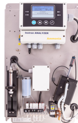
Ercros SA and Electroquímica de Hernani are two of the leading companies in the chlor-alkali industry in Spain. Both companies installed the Instran™ analyzer to monitor in real-time ammonia/ ammonium levels in brine.
