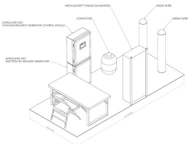
SafeGuard™ H2O Cr6 Removal Demonstration Trailer comprises five main components: the stannous reagent generation control module, electrolytic reagent generator, contactor, sand media filter and the MetalGuard™ online Cr6 monitor.
