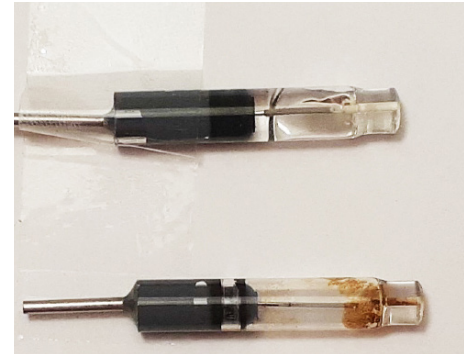
Effect of the sample quality on the probe condition - Top: healthy probe; Bottom: fouled probe.
