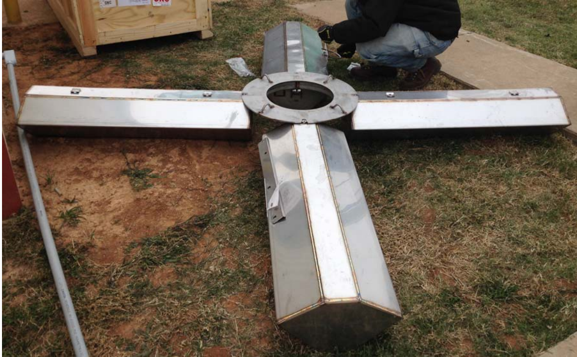
Figure 2-6 Photo of the surface aeration float used for demonstration testing
