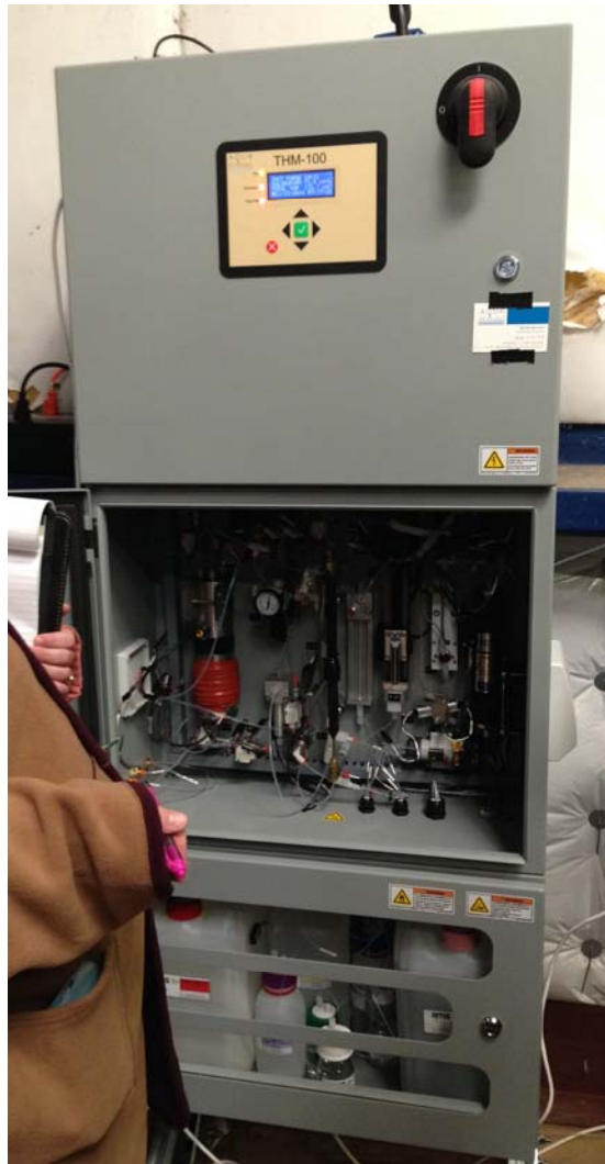
Figure 2-8 Photo of the AMS THM 100™ analyzer used for demonstration testing
