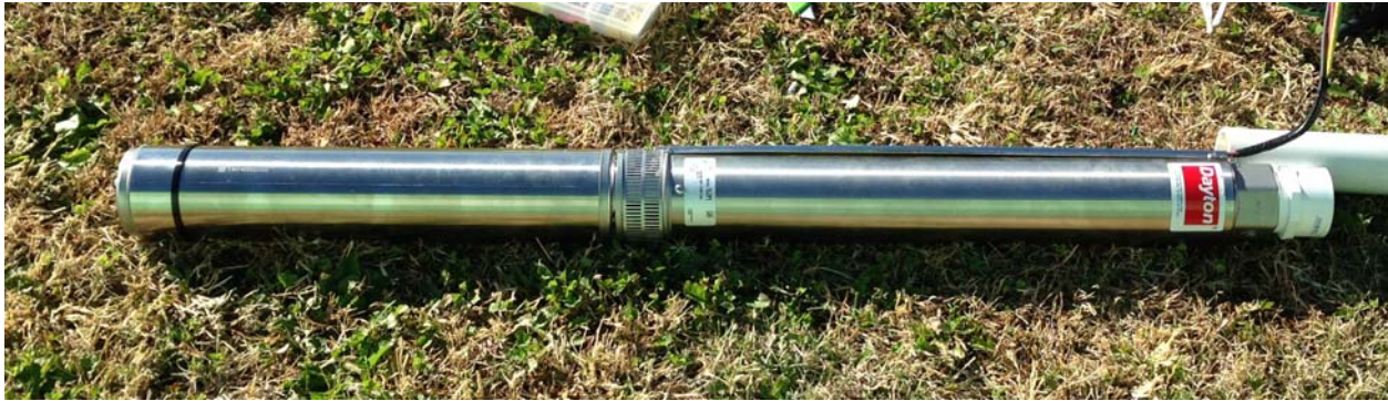
Figure 2-4 Photo of the spray aeration pump used for demonstration testing
