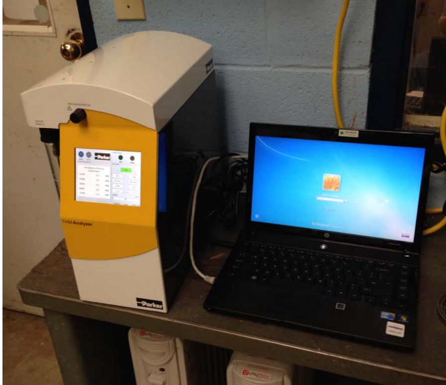
Figure 2-9 Photo of the Parker THM analyzer used for demonstration
