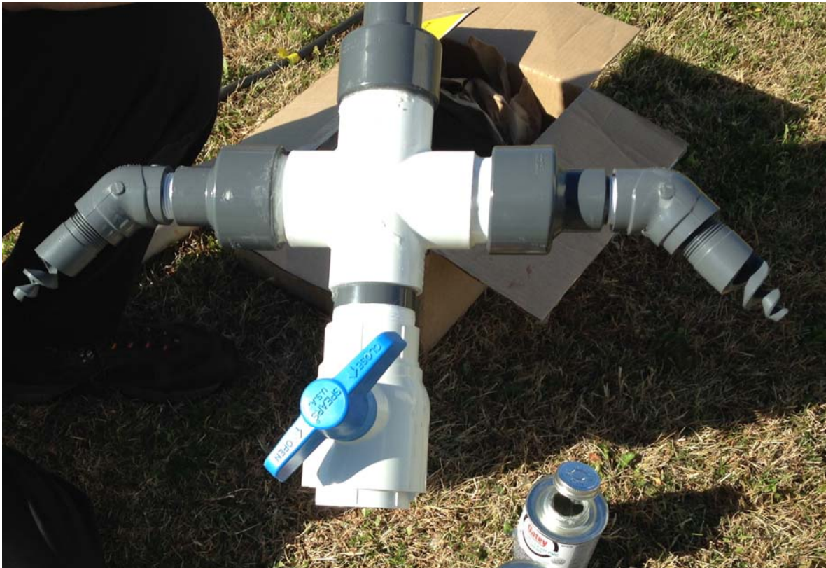
Figure 2-5 Photo of the spray aeration nozzles used for demonstration testing
